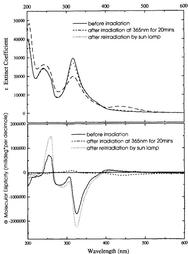
Fig. 9. Absorption (upper) and ICD (bottom) of 5 vesicles before and after irradiation.
